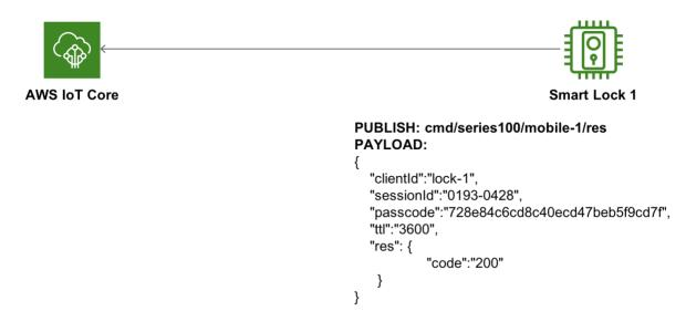
Figure 10: Smart lock response published to AWS IoT Core
