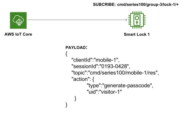
Figure 9: Command sent from the AWS IoT Device Gateway to the smart lock
