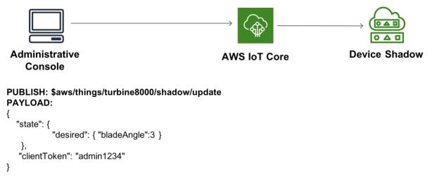
Figure 5: Command request to wind turbine device shadow
