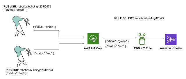
Figure 4: Many-to-one communication in fan-in pattern
