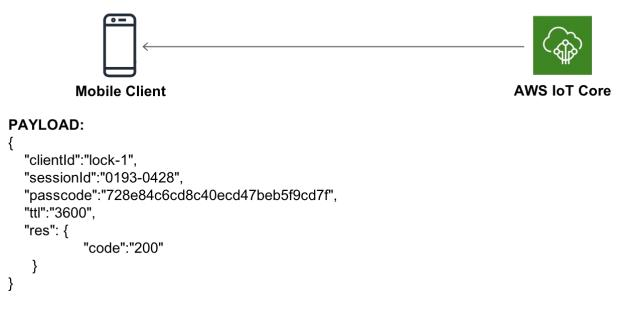
Figure 11: Command response sent from AWS IoT Core to mobile client
